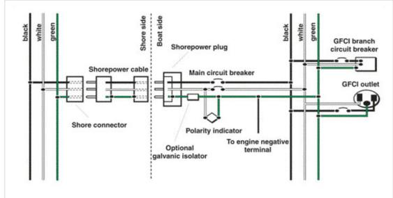
Figure 2. Ground fault circuit interrupters (GFCI) should be installed in each AC circuit. A GFCI will disconnect power in the presence of ground currents, helping prevent an electrocution.
