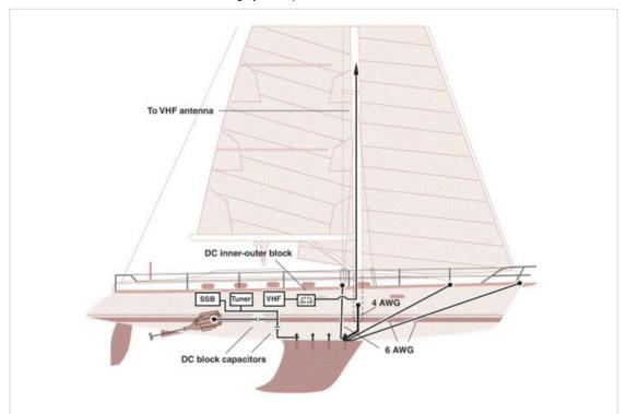
Figure 3. Conductors running from the external keel or ground plate to the mast, stays and to the metal fuel tank will protect against a lighting strike, and there will be no DC connections to the engine or to the electrical system.
